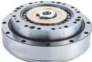
RHSG-II is standard hollow hat shaped harmonic reducer, with compact structure. The input shaft is connected to the wave generator's inner hole through an Oldham coupling. Generally, the circular spline end will be fixed, and the flex-spline end is the output.
