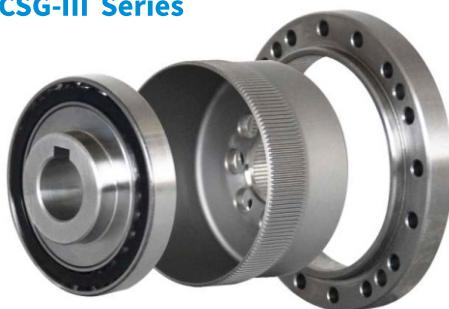
RCSG-III is composed of three parts: a flexspline, a rigid circular spline, and a wave generator. The flexspline is standard cup-shaped structure. The input shaft is directly matched with the wave generator's inner bore by flat key or screws.
