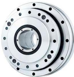
RHSG-III is standard hollow hat shaped harmonic reducer, with compact structure. The wave generator's center is a hollow shaft, the reducer inside designed with bearing support. This model is very suitable for threading. The fully sealed structure is easy to install.
