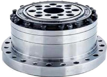
RCSG-I is standard cup-shaped structure. The input shaft is directly matched with the wave generator's inner bore by a flat key. Generally, the circular spline end will be fixed, and the flex-spline end is the output.
