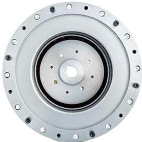
RHSG-I is standard hollow hat shaped harmonic reducer, with compact structure. The input shaft is directly matched with the wave generator's inner bore by a flat key. Generally, the circular spline end will be fixed, and the flex-spline end is the output.
