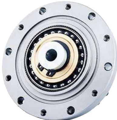
RCSG-II is standard cup-shaped structure. The input shaft is connected to the wave generator's inner hole through an Oldham coupling. Generally, the circular spline end will be fixed, and the flex-spline end is the output.
